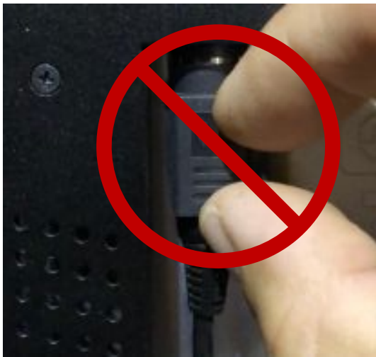
Locked position - Don't pull out
